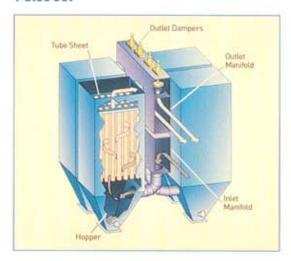
In the pulse jet cleaning process, a pulse of high pressure air is forced downward through the bag causing the dust layer formed on the outside of the filter media to release and fall into the hopper. The advantage of pulse jet cleaning is that the filtration process does not have to stop in order for cleaning to take place and higher air to cloth ratios are possible.
